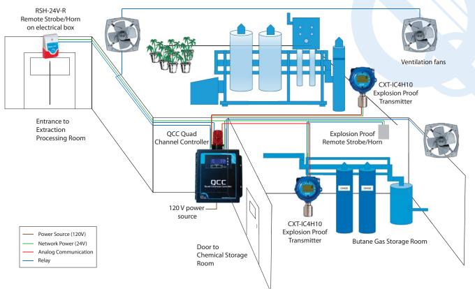
Inside the oil extraction processing area, a CXT-A-IC4H10 Explosion Proof transmitter with an infrared Butane sensor should be mounted 6 inches from the floor near the extractor and where the gas is likely to collect. Butane is heavier than air and will collect in low places. Outside the door of the extraction processing area door should be an audible/visual alarm device such as the RSH-24-R Remote Strobe / Horn.
