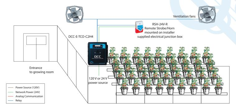
The DCC-E-TCO-C2H4 Dual Channel Controller with an internal Carbon Monoxide sensor and internal Ethylene sensor should be mounted in the greenhouse where the plants are growing. Both gases are close to the same weight as air and will hang around in the "breathing zone" so the DCC should be mounted (1.2 m - 1.8 m / 4 - 6 ft) from the floor.
